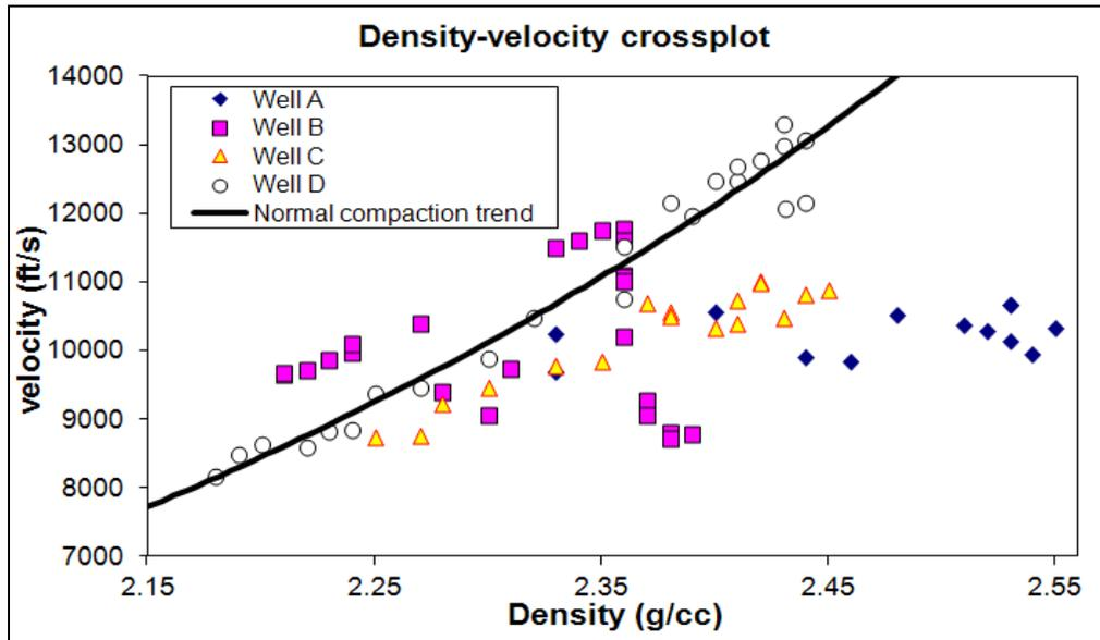
**Figure 5:** Density versus Velocity crossplots for the Onshore Niger Delta study wells.
