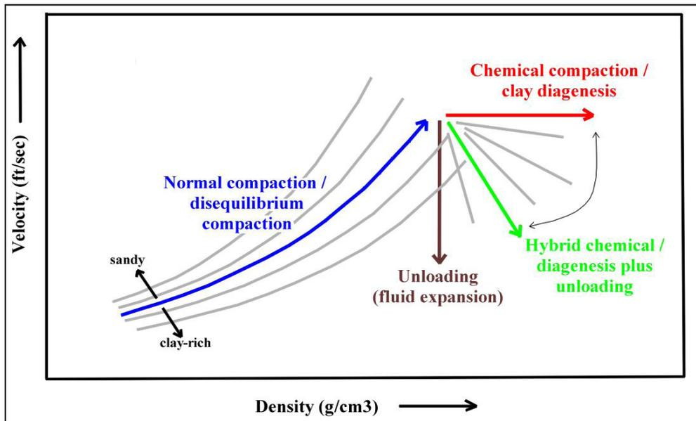
**Figure 4:** Typical Hoesni curve-types from Velocity-Density crossplots with associated overpressure generating mechanisms. (Source: O'Connor et al., 2011).
