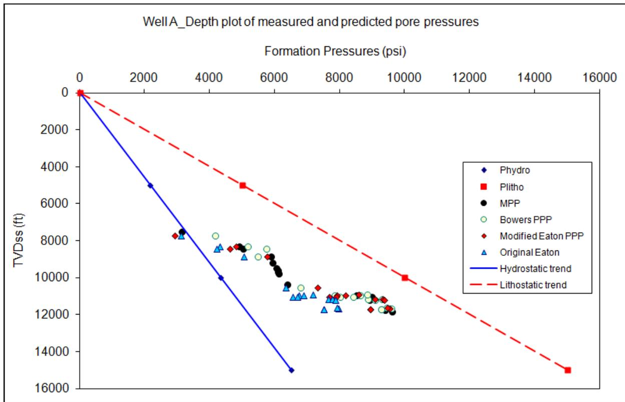
**Figure 8:** Comparison of Measured and 1D Predicted Pore Pressures for Well A. Original Eaton exponent under predicts formation pressures in the deeper sections of the well whereas modified Eaton yields a good match.
