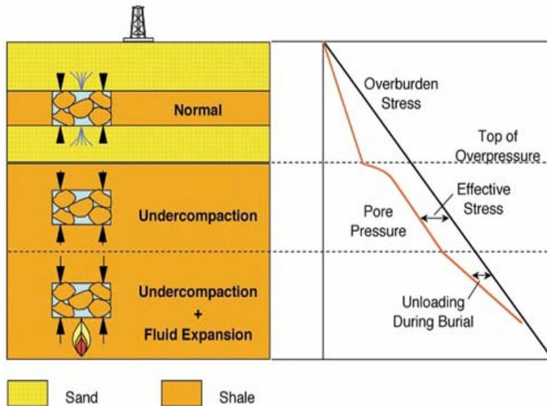
**Figure 2:** Pressure trends and response of vertical effective stress to different overpressure-generating mechanisms (source: Bowers, 2002)
