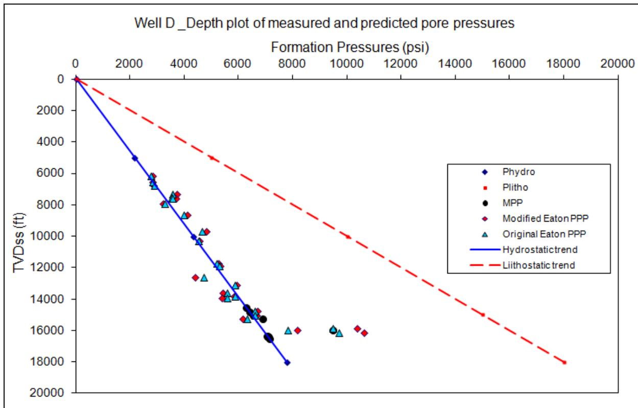
**Figure 11:** Comparison of Measured and 1D Predicted Pore Pressures for Well D
