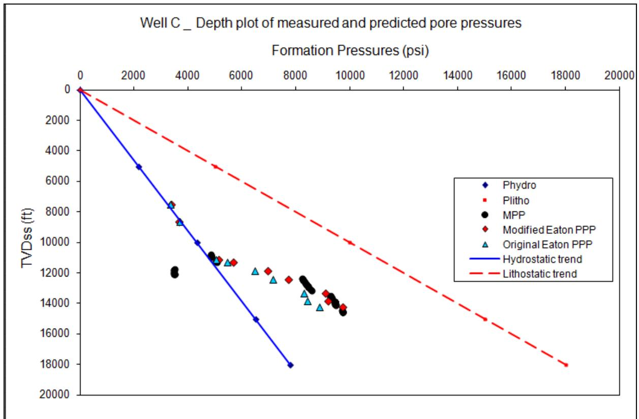
**Figure 10:** Comparison of Measured and 1D Predicted Pore Pressures for Well C
