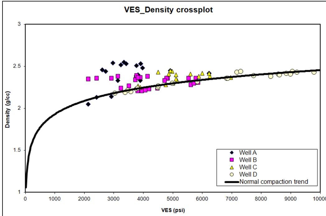
**Figure 7:** Crossplot of Vertical Effective Stress and Density for the wells. Deep section data in both well A and B trend as reversals away from the normal compaction curve.
