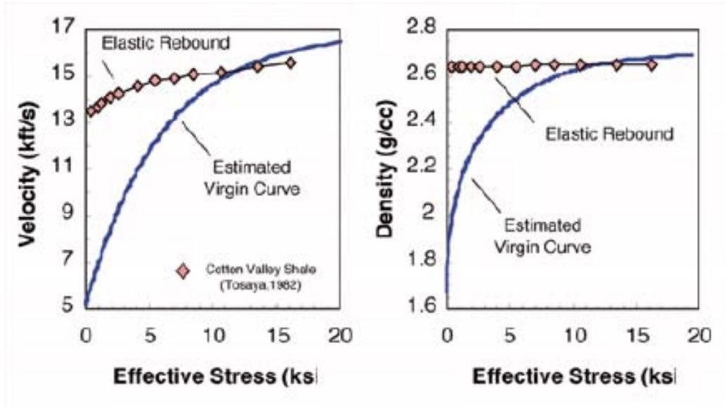
**Figure 3:** Typical VES-Velocity and VES-density signatures for shales in unloading situations (source: Bowers, 2002).
