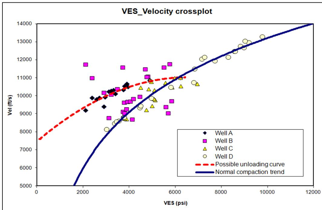
Figure 6: Crossplot of Vertical Effective Stress and velocity data for the wells. Note the unloading limb (black dots and red dotted line) established by well A data and closely followed by data points from deep sections of well B.
