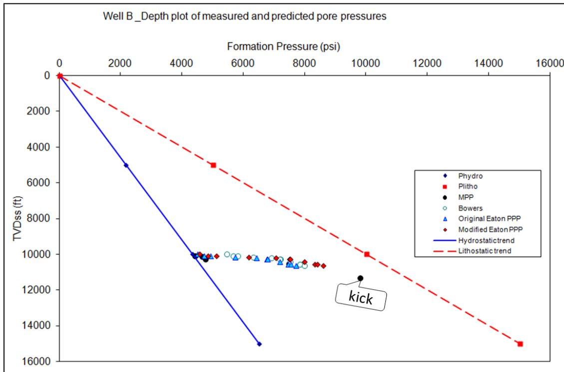
**Figure 9:** Comparison of Measured and 1D Predicted Pore Pressures for Well B.
