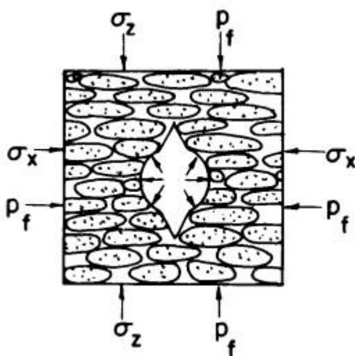
**Fig. 8** Underground stress distribution showing fluid cavity which can initiate hydraulic fracturing (Pressure > Pore Pressure) (<sup>2</sup>)
