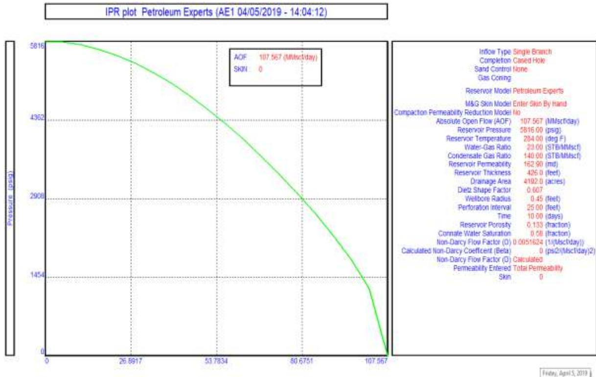
**Figure 6** IPR Curve for gas condensate reservoir.
