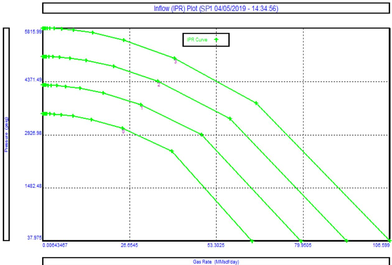
**Figure 7.** Effect of reservoir pressure on Future IPR.
