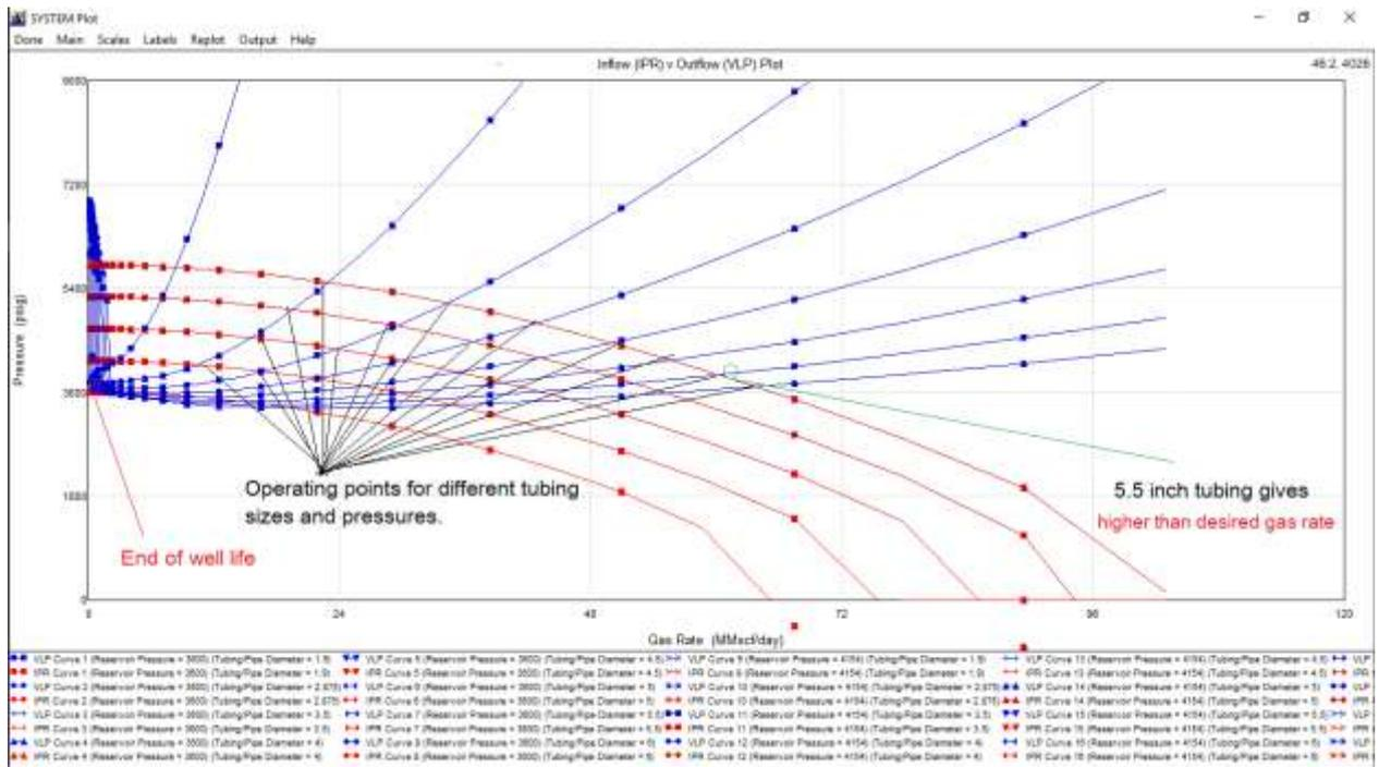
Figure 8 Different tubing sizes analysis (Hagedorn Brown)
