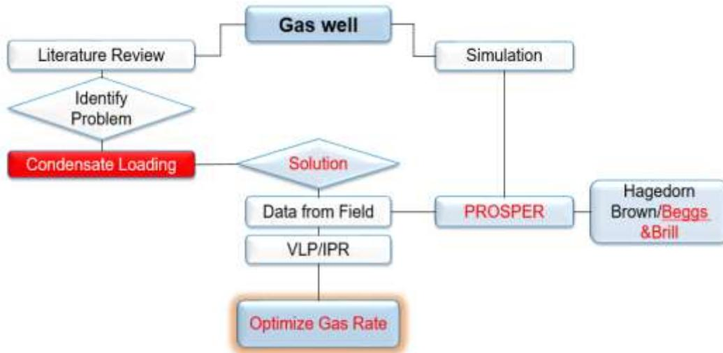
Figure 3 Flow diagram of the Gas condensate well optimization process
