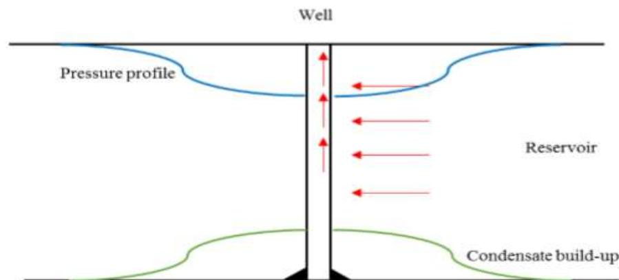
**Figure 1.** Condensate buildup in the near-wellbore area (after Baker 2005)
