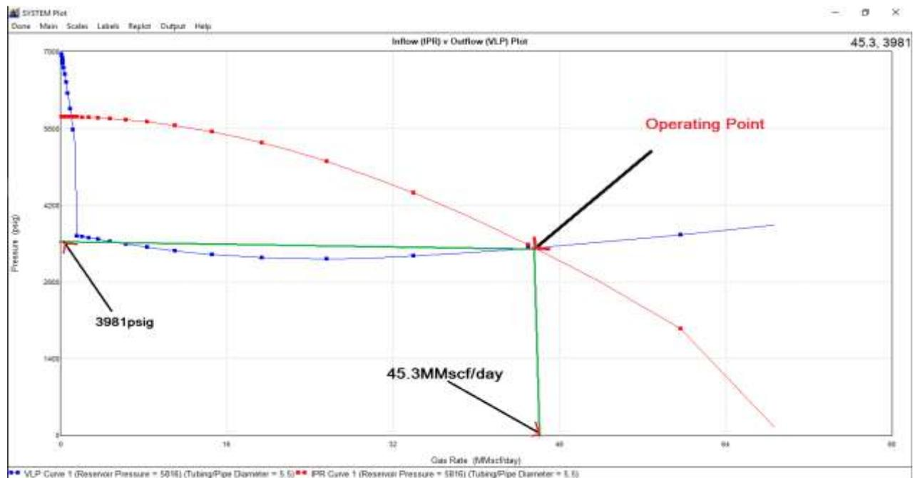
**Figure 10** Inflow (IPR) Vs. Outflow (VLP) Plot for 5.5in tubing.
