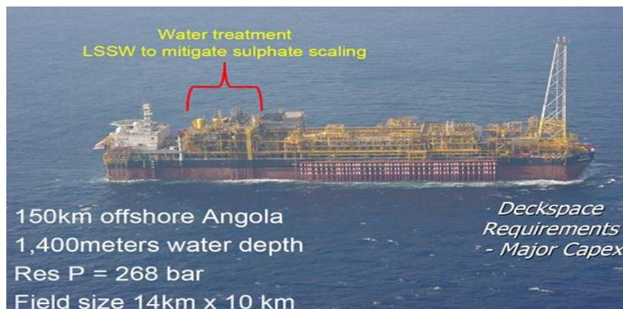
**Figure 5:** Grrasol Angola; Water treatment to mitigate sulphate scaling.
