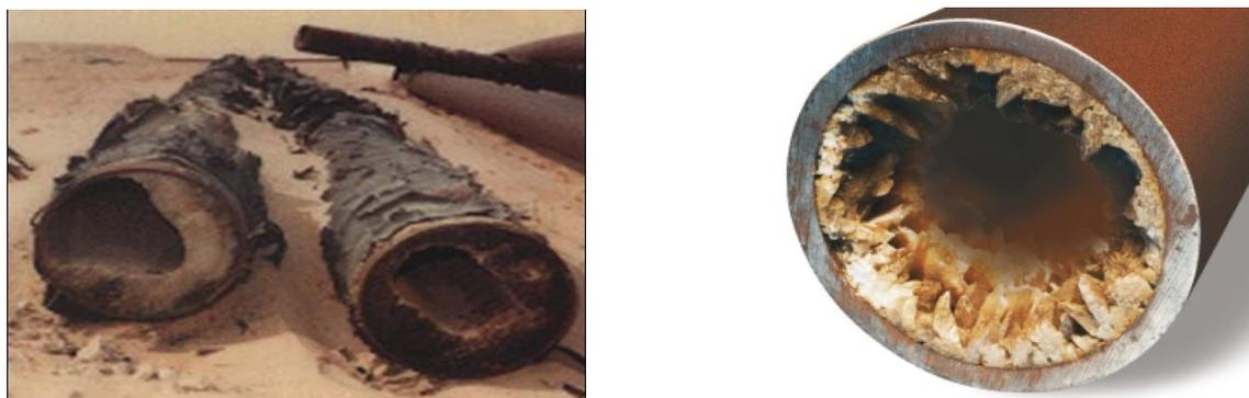
**Figure 1:** Severity of scale deposits in oilfield equipment before inhibitions treatment<sup>2</sup>
