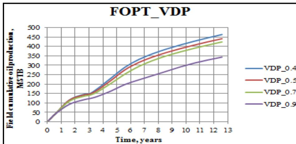
**Figure 17:** Plot of field cumulative production vs. time for all  $V_{DP}$  scenarios.
