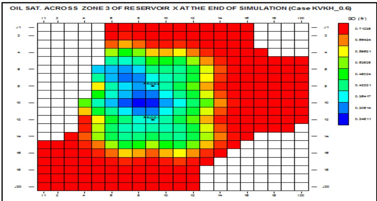
**Figure 11:** Map showing the distribution of oil saturation across zone 3 of the Reservoir X and the location of producers at the end of simulation (01/01/2009) for kV/kH case KVKH\_0.6.
