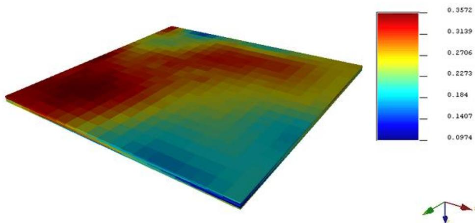
**Figure A3:** Simulation map showing porosity distribution across the Reservoir X model.
