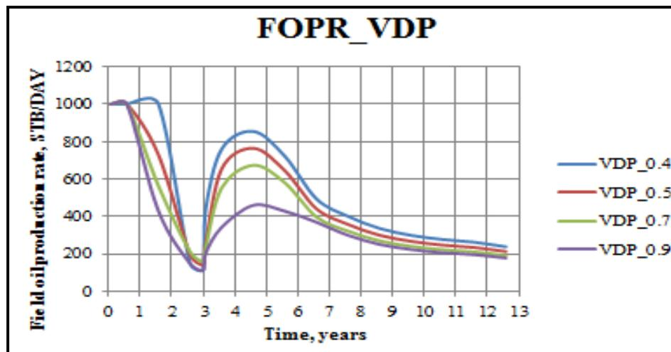
**Figure 15: Plot of field oil production rate vs. time for different  $V_{DP}$  scenarios.**
