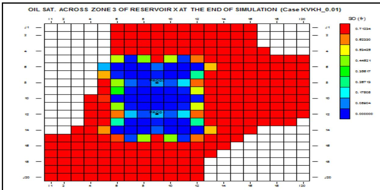
**Figure 9:** Map showing the distribution of oil saturation across zone 3 of the Reservoir X and the location of producers at the end of simulation (01/01/2009) for kV/kH case KVKH\_0.01.
