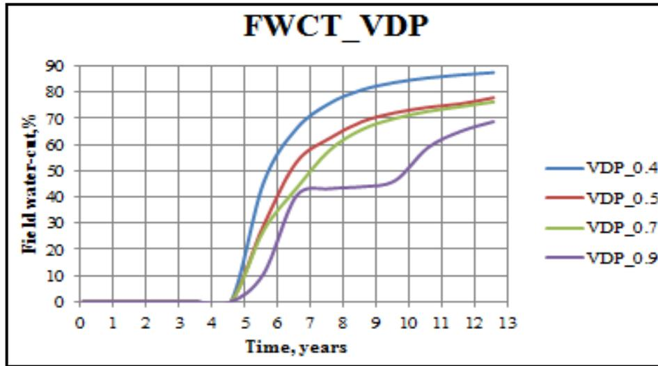
**Figure 16:** Plot of field water-cut vs. time for different  $V_{DP}$  scenarios.
