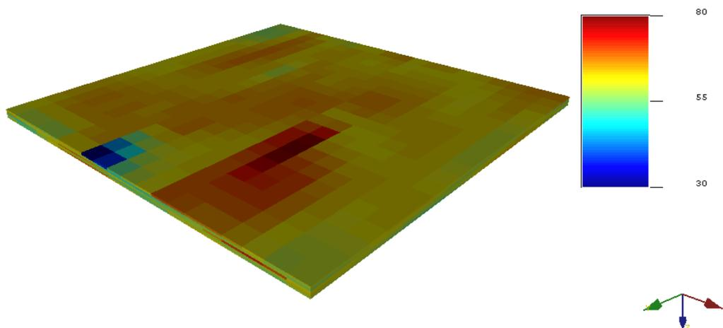
**Figure A4:** Simulation map showing net-to-gross distribution across the Reservoir X model.
