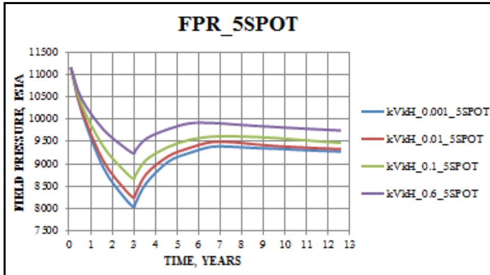
**Figure 13:** Plot of field pressure vs. time for different  $k_V/k_H$  ratios.
