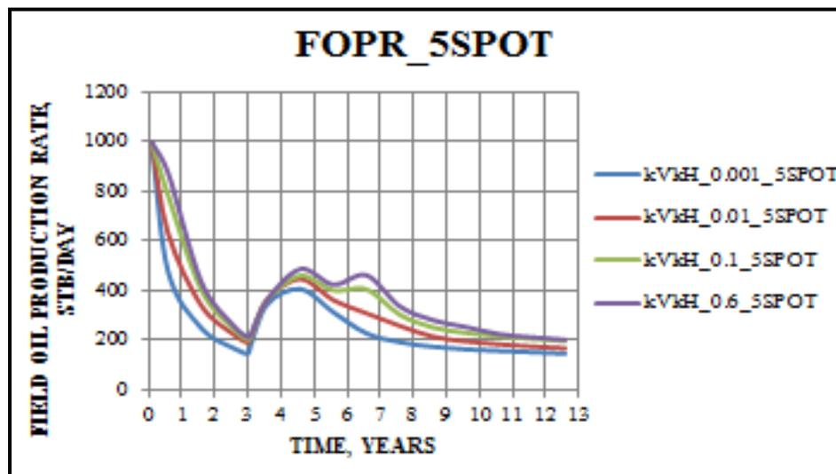
**Figure 7:** Plot of field oil production rate vs. time for different  $kV/kH$  ratios.
