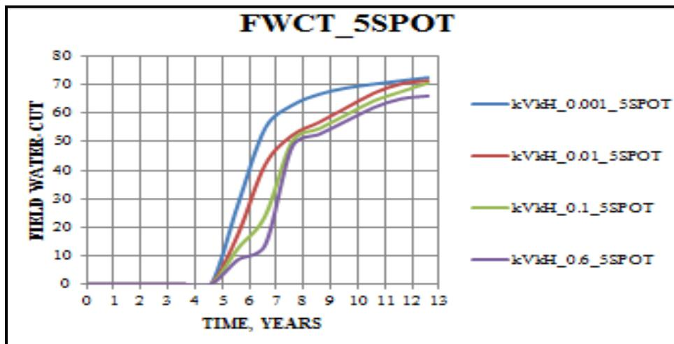
**Figure 14:** Plot of field water-cut vs. time for different  $k_V/k_H$  ratios.
