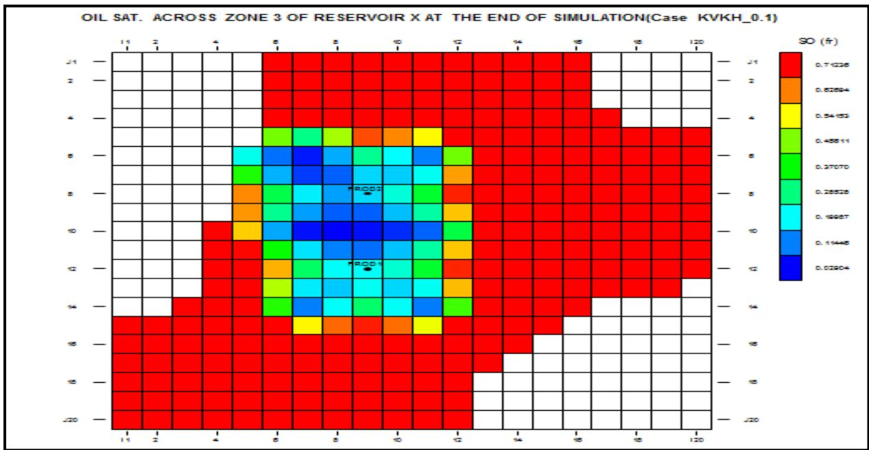
**Figure 10:** Map showing the distribution of oil saturation across zone 3 of the Reservoir X and the location of producers at the end of simulation (01/01/2009) for kV/kH case KVKH\_0.1.
