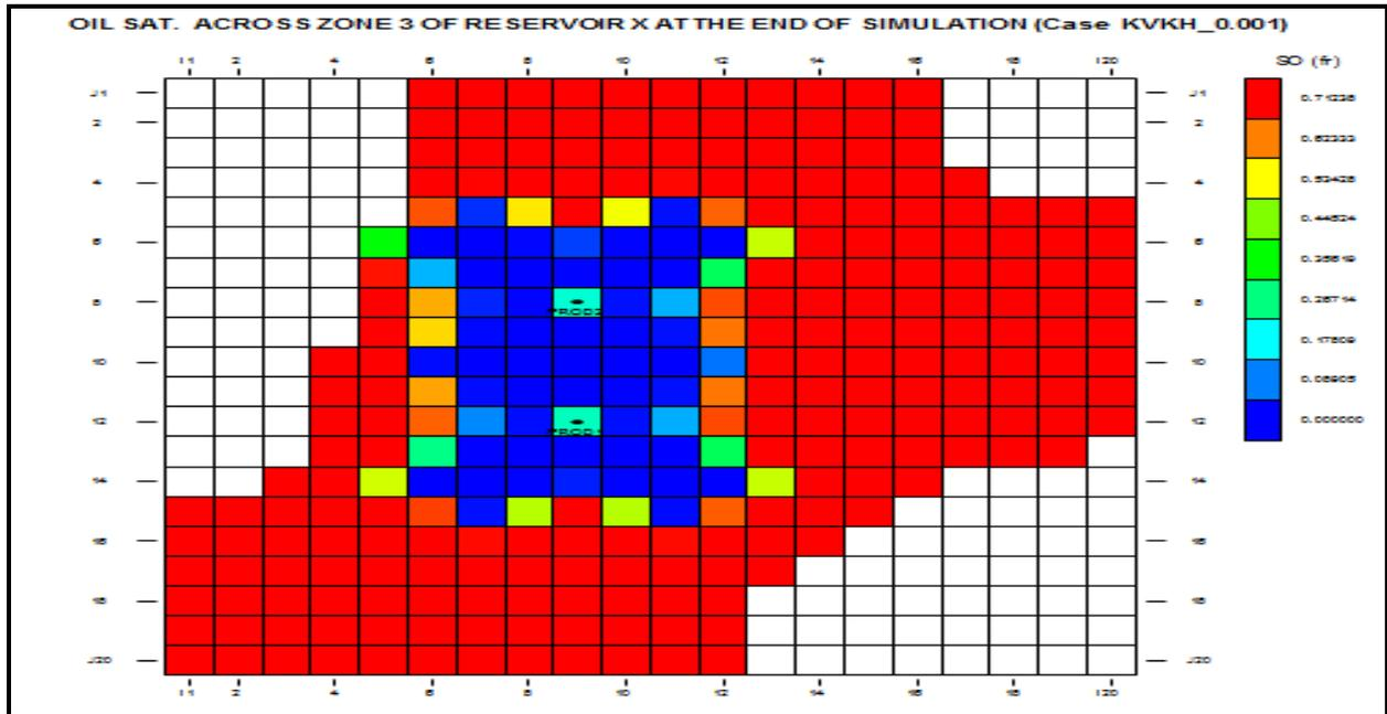
**Figure 8:** Map showing the distribution of oil saturation across zone 3 of the Reservoir X and the location of producers at the end of simulation (01/01/2009) for kV/kH case KVKH\_0.001.
