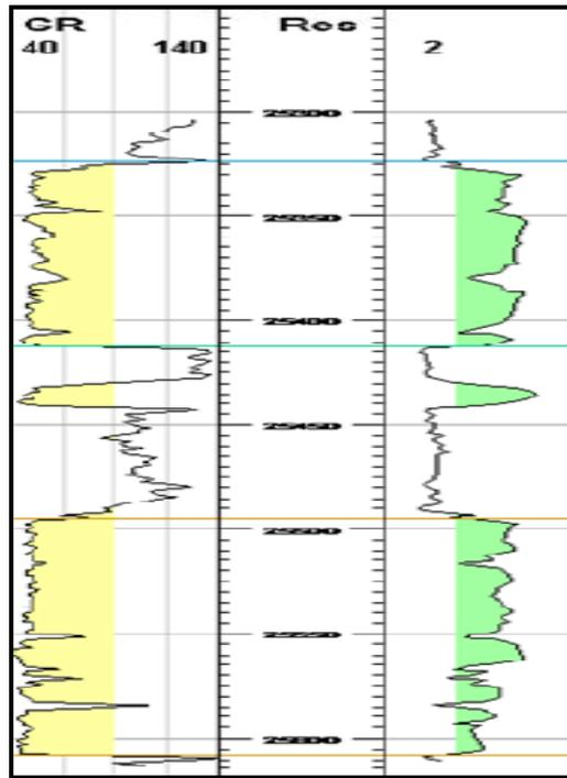
**Figure 1:** Type log of a well in the Reservoir X used to illustrate facies type (Lach<sup>10</sup>).
