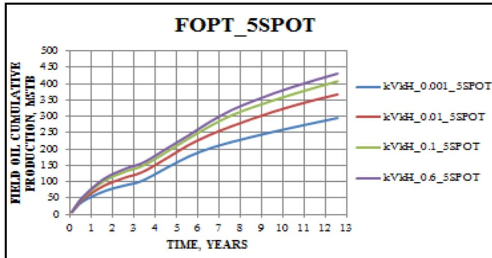
**Figure 12:** Plot of field cumulative oil production vs. time for different  $kV/kH$  ratios.
