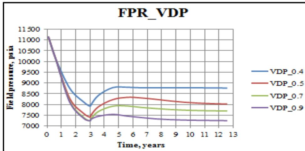
**Figure 18:** Plot of field pressure vs. time for different  $V_{DP}$  scenarios.
