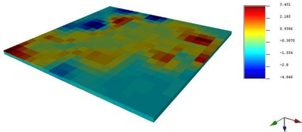
**Figure A2:** Simulation map showing permeability distribution across the Reservoir X model.
