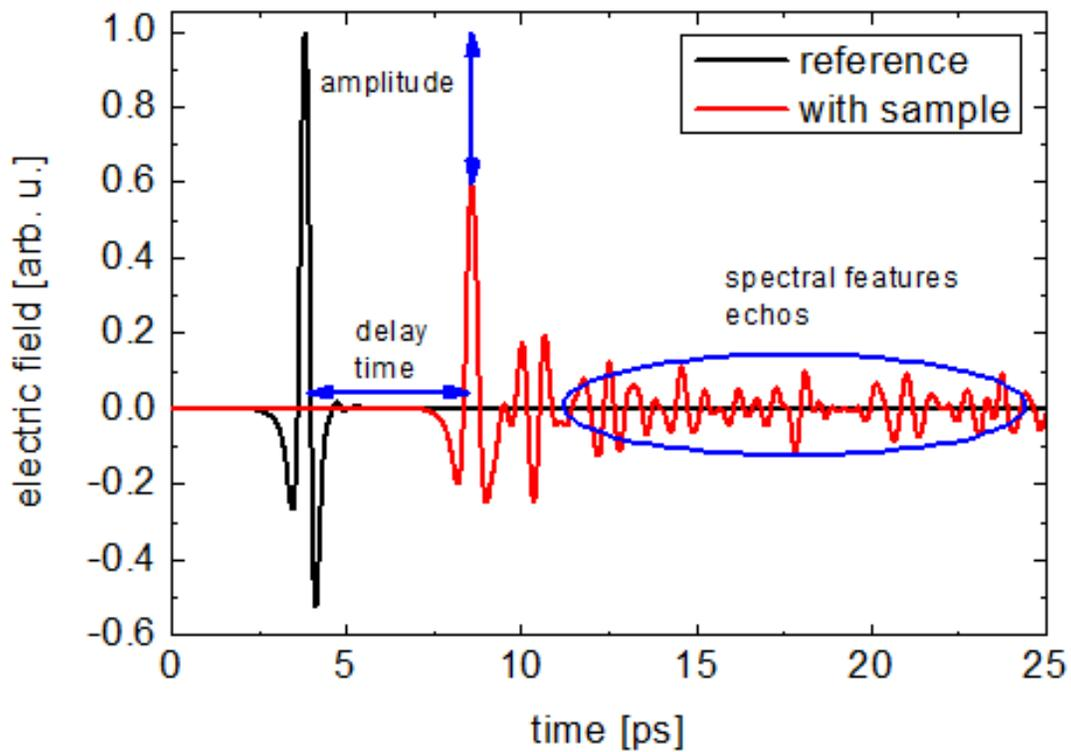
**Fig. 3.** The typically measured THz electric field signals. The reference (black) and sample (red) signal corresponds respectively to the detected THz pulse without and with the oil shale sample.
