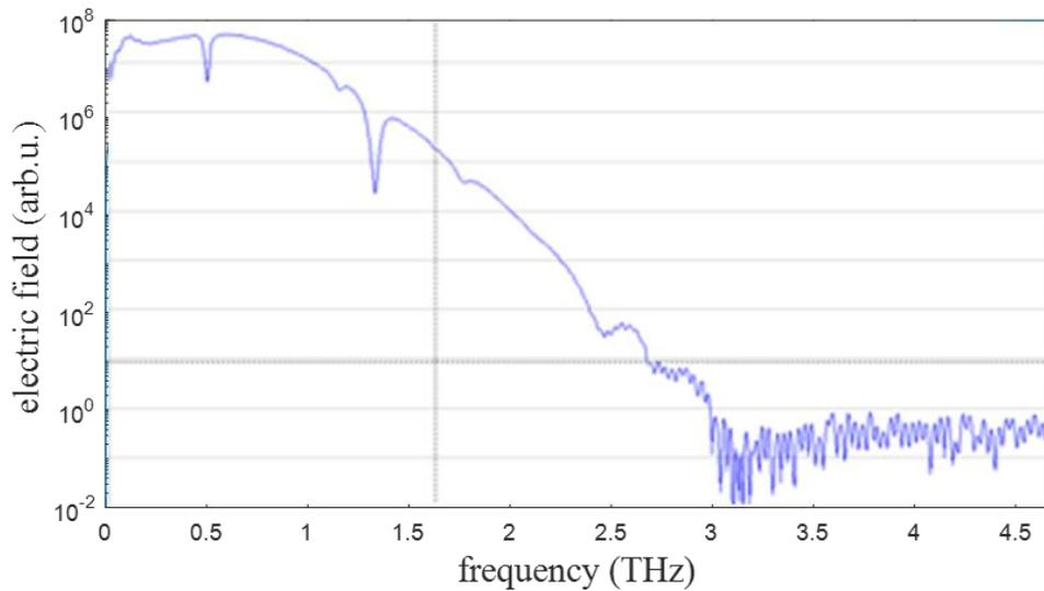
Fig. 4. A Typical spectrum plot from a THz-TDS
