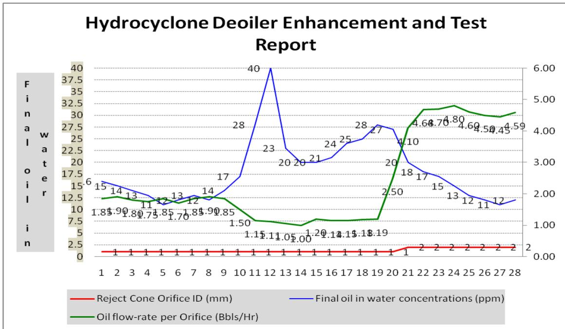
**Figure 2:** Deoiler enhancement and field performance test process parameters
