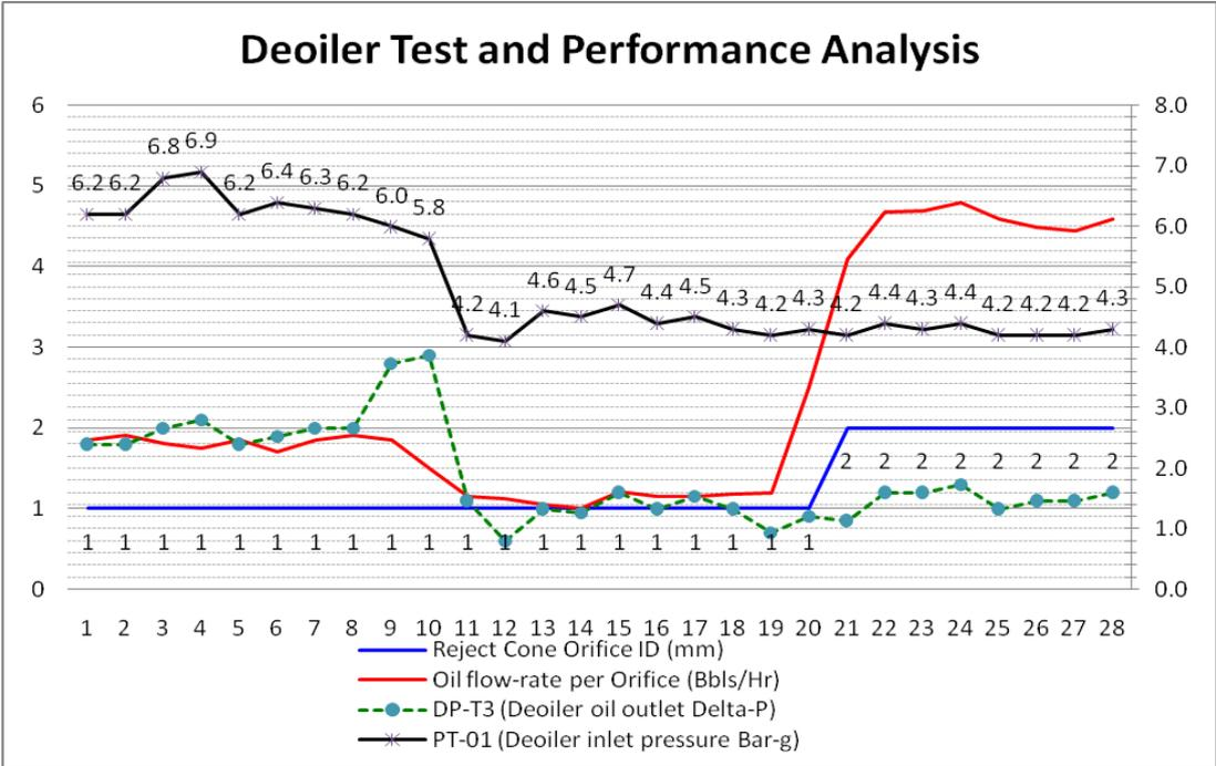
**Figure 1:** Hydro-cyclone de-oiler failure analysis and plant trail performance parameters
