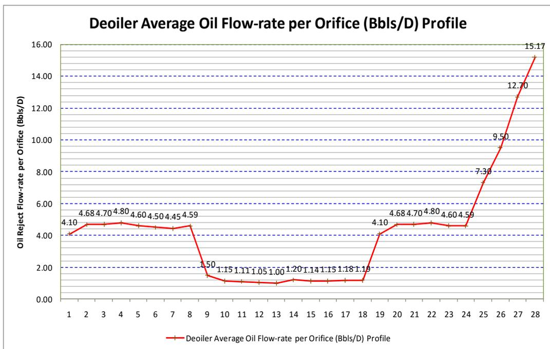
**Figure 3:** Hydro-cyclone de-oiler oil flow rate per reject cone orifice – profile
