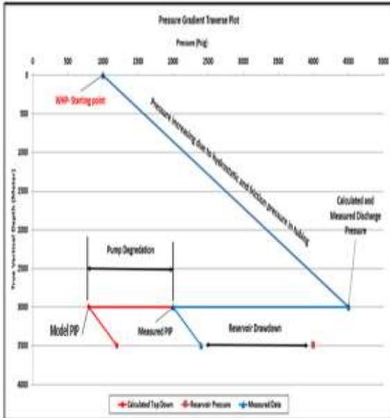
**Figure7** Unmatched Gradient traverse plot for an ESP Well
