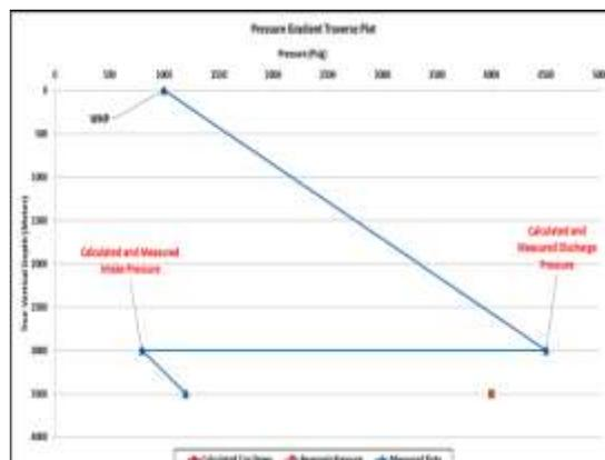
**Figure 8** Matched Gradient traverse plot for an ESP
