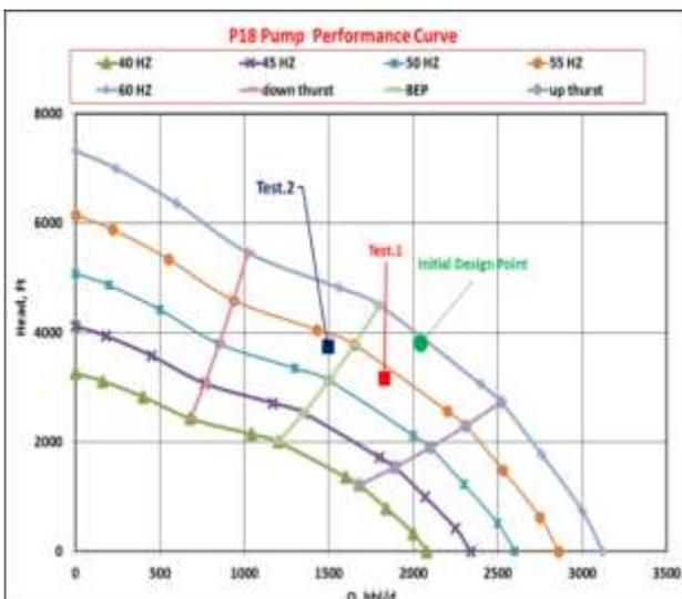
**Figure 12.** ESP performance curve of well #1
