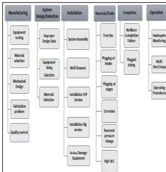
Figure 3. ESP failure causes
