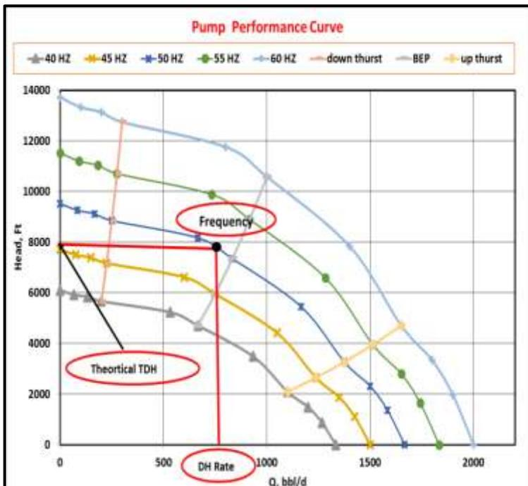
Figure 6. Determination of Theoretical TDH from Pump Curve
